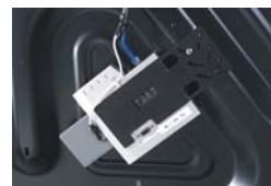
Transmitter & Antenna Discreetly trunk-mounted for wireless Ethernet data transfer
